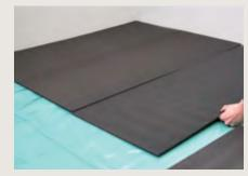
QUICKHEAT INSULATION PLATES Insulation plates.  $120 \times 50 \times 0.7$  cm. 10 plates/pack.  $0.6\text{m}^2/\text{plate}$ ,  $6\text{m}^2/\text{pack}$ . Thickness: 7 mm. Use of vapour barrier is recommended. Place PE film PGUDLSCREEN34 under QuickHeat insulation plates as well as on top of QuickHeat foils.
